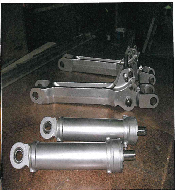
Canberra main undercarriage overhauled, hydraulic cylinders reconditioned and struts repaired
